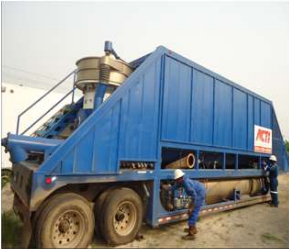
Non-man Entry Automated Tank Cleaning System (NEATS)
