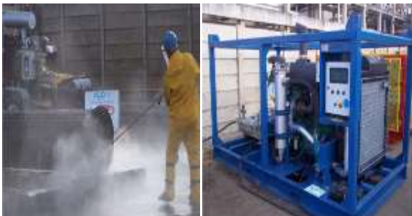
High Pressure Jetting System
